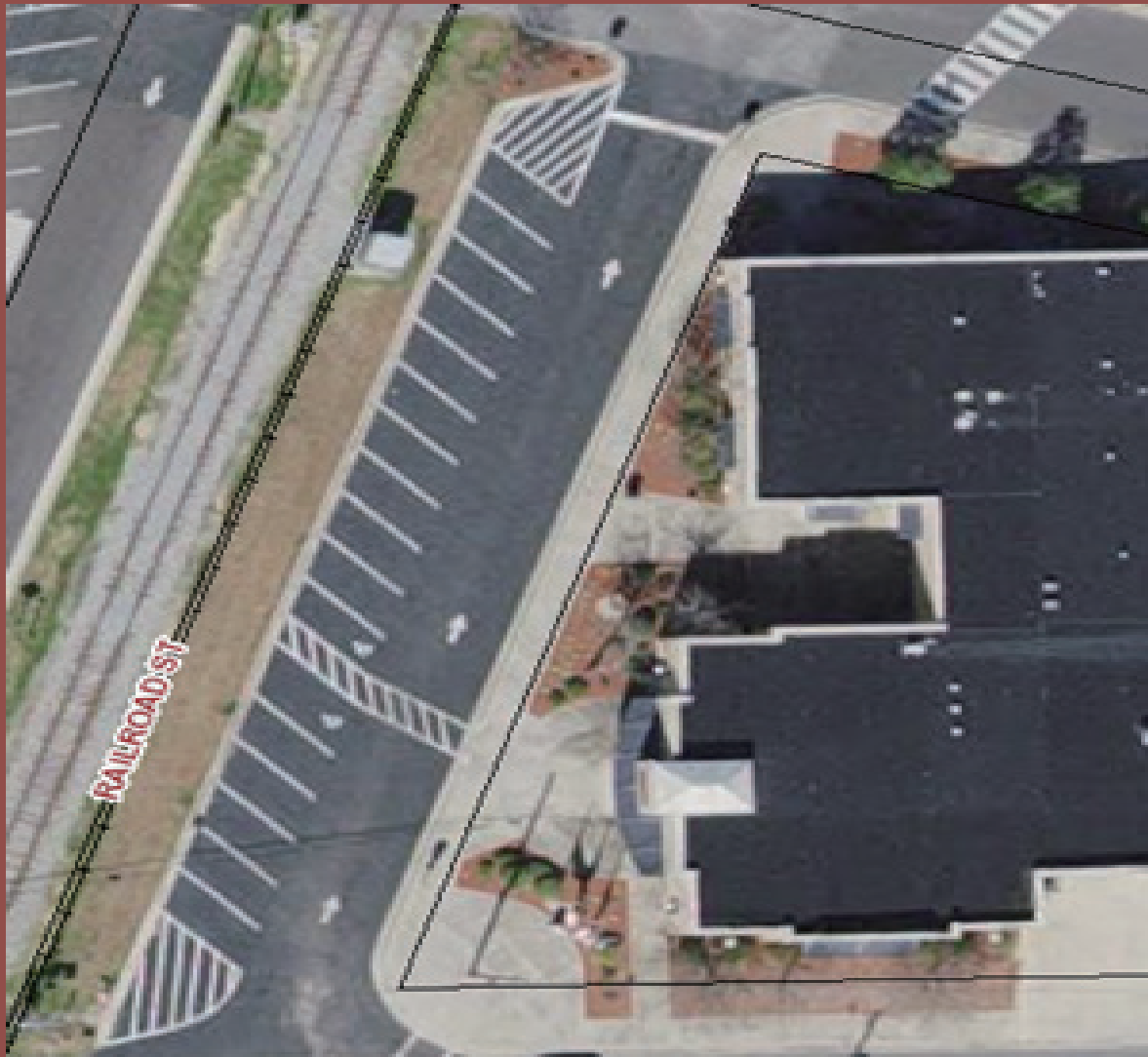
Figure #13 Angled parking in Winterville, NC Source: Pitt County OPIS Satellite imaging.
